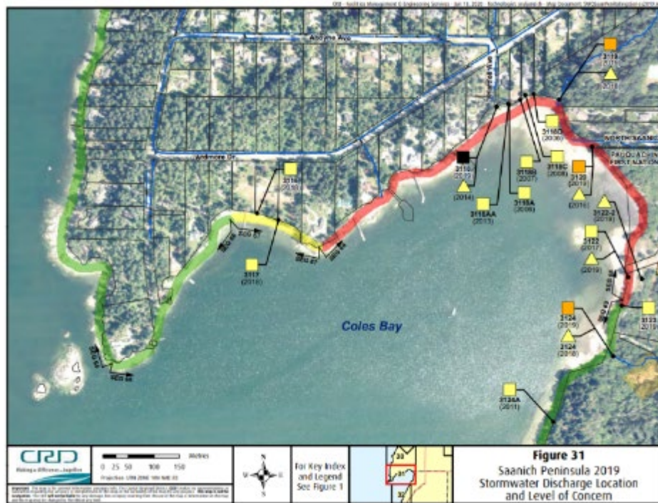
FIGURE 7: Coles Bay Storm Water Discharge and respective levels of contamination concern. 47
